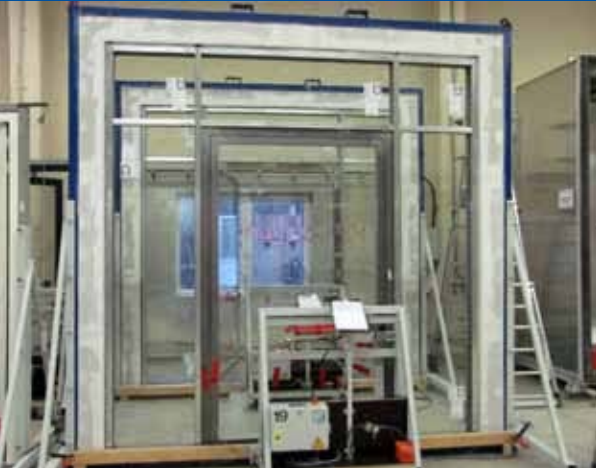
Long-term endurance test to EN 1191
